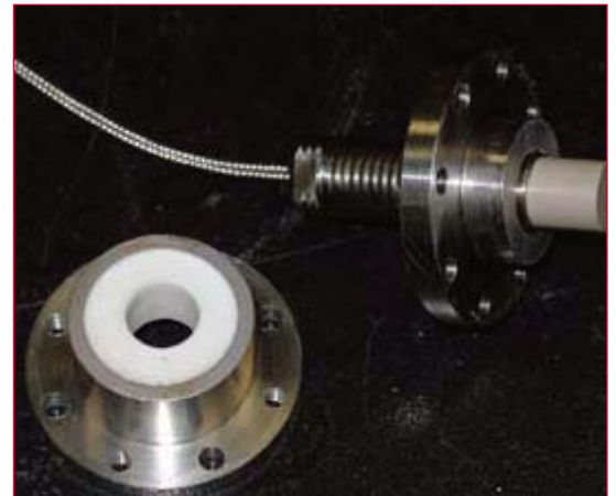
Figure 7 The sensor pocket machined to allow direct line of sight from the sensor to the blade tip
